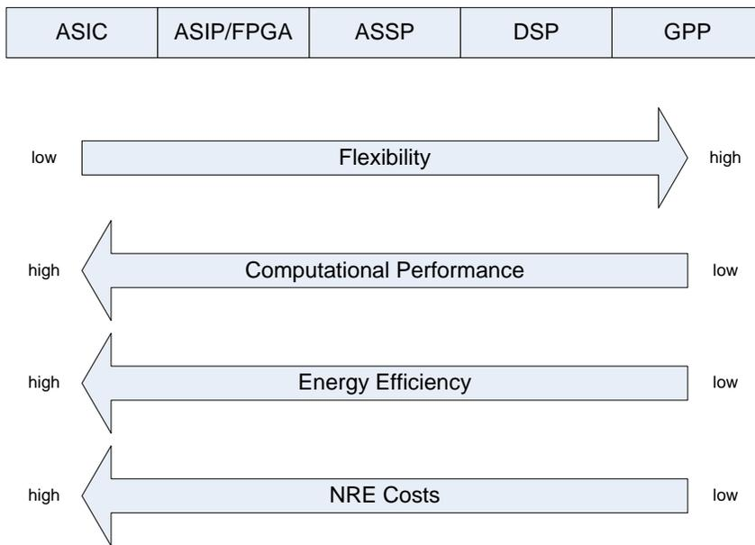
Figure 1 - Relative relations of the 5 main technologies (based on [3] and [4] with addition of NRE)
